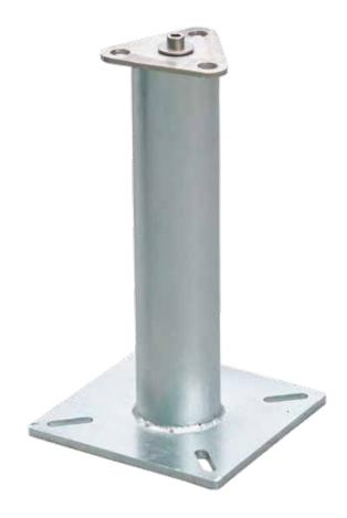
Anchor post PROTON 1 can be installed on roofs, terraces, platforms and beams. It is fitted with a three-hole plate enabling connection of personal fall protection equipment. The device complies with EN 795 type A.
