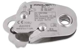
Guided type fall arrester AC 081 intended for use with polyester work rope AC 300, 12mm dia. The arrester should be connected to full body harness by an oval connector, e.g. AZ 011. Maximum load 120kg (EN 12841 as access rope).
