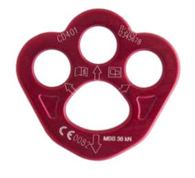
Rigging plate is designed for quick setting up of complex rigs thanks to numerous boreholes for connectors. Rigging plate has a large single main connecting point and three holes 20mm dia for connectors.
