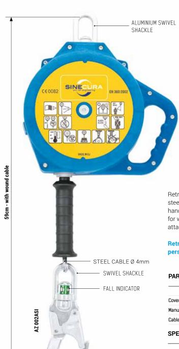
Retractable type fall arrester CR 240 with expandable steel cable in plastic cover. Fitted with a comfortable side handle. Cable diameter is 4mm. The device is intended for works requiring significant mobility in respect to attachment point. Energy absorber is not required.
