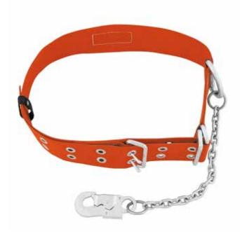
Work positioning belt PB 60 is made from a single polyester webbing strip connected by an aluminium buckle. Fitted with a welt to enable smooth belt length adjustment (length between 0.45m and 2.0m). Chain with steel connector AZ 002 at the end.Work positioning belt PB 60 complements fall protection equipment and prevents falls during works at height.
