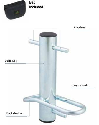
Port-a-wrap - TU 100 - a device designed for arborists. Used mainly for sectional tree felling. Used for controlled descending of material. By correct weaving the cable through the device, branches or parts (sections) of the trunk can be safely lowered to the ground. Maximum tree diameter for cargo lashing AX 500 is 1.2m.
