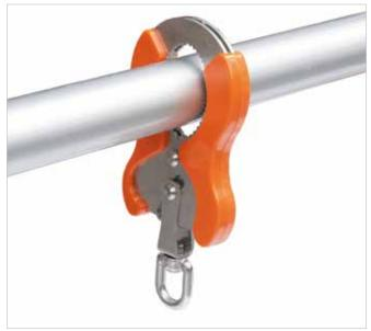
Anchor device AZ 300 is intended for use by one person; to be used as a protection against falls from a height when working on scaffolds. To be used on tubes, 44.5 - 50mm dia.
