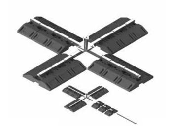
Deadweight IM 200 is a portable anchor point for use on a flat roof of adequate load capacity. Comprises 12 elements (weights) and the main cross piece with mounted pole PROTON I (300mm). The IM 200 device should be placed so that it rests firmly on the roof surface.
