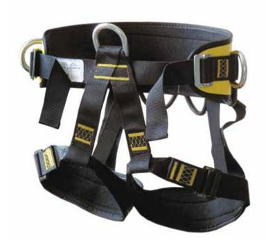
Belt fitted with ergonomically profiled padding, connecting and adjusting buckle, side attachment buckles and attachment point for work in a harness. Work positioning belt / sit harness PB 70 complements fall protection equipment and prevents falls from height during works at poles, trees, building structures, etc.
