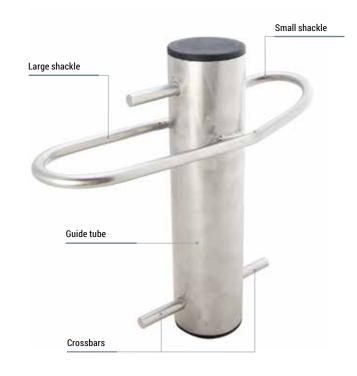
Port-a-wrap - TU 201 - a device designed for arobrists made of stainless steel. Used mainly for sectional tree felling. Used for controlled descending of material. By correct weaving the cable through the device, branches or parts (sections) of the trunk can be safely lowered to the ground.
