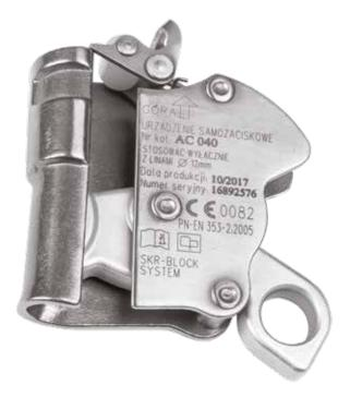
Guided type fall arrester SKR-BLOCK intended for use with polyester work rope AC 200, 12mm dia. The device should be connected to full body harness by an oval connector, e.g. AZ 011.
