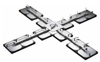
Deadweight IM 100 is a portable anchor point for use on a flat roof of adequate load capacity. Comprises 12 elements (weights) and the main cross piece with anchor point. The IM 100 device should be placed so that it rests firmly on the roof surface.
