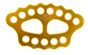
Rigging plate enables perfect alignment of connectors in the line of action of the force. It can also be used as a main rigging point in complex systems. The rigging plate has 5 holes 20mm dia at one side, and 8 holes 20mm dia for connectors.
