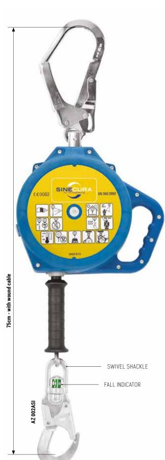
Retractable type fall arrester CR 241 with expandable steel cable in plastic cover. Fitted with a comfortable side handle. Cable diameter is 4mm. The device is intended for works requiring significant mobility in respect to attachment point. Energy absorber is not required. The arrester is equipped with fixed connector AZ 022.
