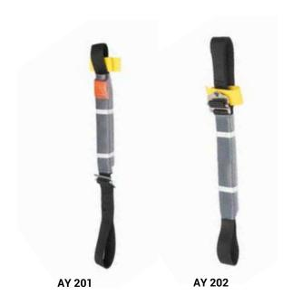
Trauma strap AY 201 and AY 202 is designed to alleviate the effects of suspension trauma on a worker who has fallen in full body harness. It can be attached to full body harness and enables shifting the worker's body weight onto the leg.
