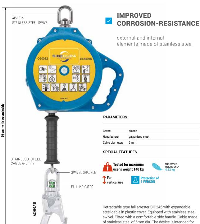
Retractable type fall arrester CR 245 with expandable steel cable in plastic cover. Equipped with stainless steel swivel. Fitted with a comfortable side handle. Cable made of stainless steel of 5mm dia. The device is intended for works requiring significant mobility in respect to attachment point. Energy absorber is not required. Retractable type fall arrester CR 245 is a component of personal fall protection equipment.
