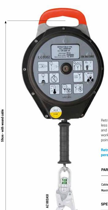
Retractable type fall arrester CR 220 with expandable stainless steel 5mm cable. Mechanism is made of stainless steel and enclosed in plastic cover. The device is intended for works requiring significant mobility in respect to attachment point. Energy absorber is not required.
