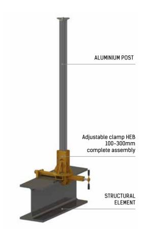
Proton 6 is an anchor point for individual fall protection equipment. Proton 6 can be installed on HEB I-beams, 100mm to 300mm wide. The device is made of a strengthened aluminium alloy and stainless steel.
