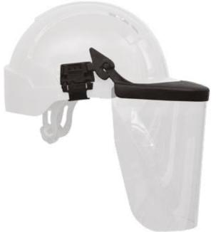
Provides protection against particles of moderate energy and moving at 120m/s, and liquid and molten metal splashes, and also arcing. Optical properties of the shield meet requirements of optical class 1 (the highest).
