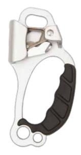
Handled ascender CD 211 and CD 212 with handle for right- and left-hand users is designed for rope ascending on vertical surfaces or on slopes. To be used with a kernmantle rope 8-13mm dia. Fitted with rope grab.
