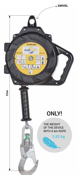
CR 250V self-locking device for vertical operation in a plastic casing with a pull-down steel rope and a swivel mounted in the casing. The device is designed for work requiring significant displacement in relation to the point of attachment. No need to use a shock absorber.
