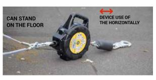
CR 250H + V self-locking device for vertical and horizontal operation in a plastic casing with a pull-down steel rope and a swivel mounted in the casing. The device has an additional shock-absorbing system located near the snap-hook. It is intended for work requiring considerable displacement in relation to the point of attachment. No need to use a safety shock absorber. No need to use AZ 800 cable when working horizontally.
