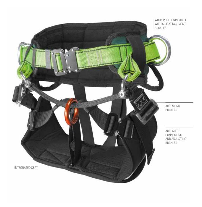
Work positioning belt for tree climbers TH 50 with an integrated seat. Equipped with ergonomically profiled padding, adjusting buckles, side attachment buckles and attachment point for work in a harness complying with EN 813. The belt includes automatic connecting and adjusting buckles Comfortable wearing and removal. Belt TH 50 is a basic equipment for works at height, mainly at trees, poles, building structures, etc.
