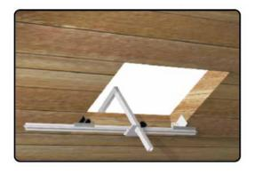
Light aluminium alloy anchor beam AT 062 with a stabilising clamp is a component of fall protection equipment and can be used as a portable anchor device. The beam can be used in building openings (windows and doors), 300 to 1270mm wide. It is fitted with two fixing plates. Beam AT 062 must be used with personal fall protection equipment.
