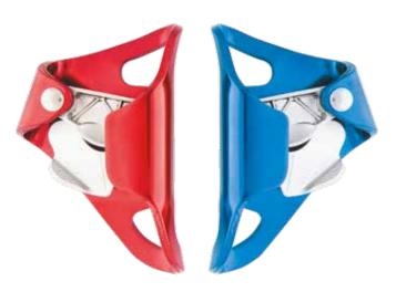
Chest ascender CD 201 ultra light and CD 202 ultra light without handle is designed for rope ascending or belaying. To be used with a kernmantle rope 8-13mm dia. Fitted with rope grab.
