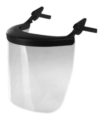
Provides protection against particles of low energy and moving at 45m/s, and liquid splashes. Optical properties of the shield meet requirements of optical class 1 (the highest). The face shield comes out with mounting clamps included.
