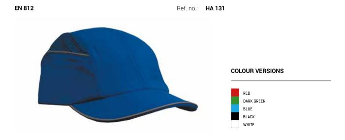
Industrial safety helmet intended for head protection against impacts by solid stable objects. Manufactured as a textile peaked cap equipped with protective pad. The cap has length-wise ventilation holes protected by polyester mesh, hard peak with polyamide pad and cotton adjustment strap at the back. Head size: 55 - 62cm.
