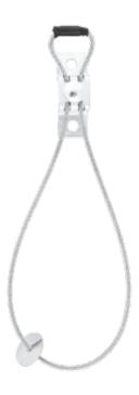
Connecting lanyard AT 192 is a component of personal fall protection equipment. The lanyard should be used as a permanent anchor device type A, enabling connection of connecting and absorbing device to a structural anchor point. Connecting lanyard is formed by a stainless steel cable, 5mm dia. Device length from 0.35 to 5.0m. Fitted with a galvanized steel handle.
