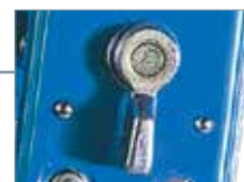
Switch for winch mechanism clutch disengagement and switching of descent/lift modes.
